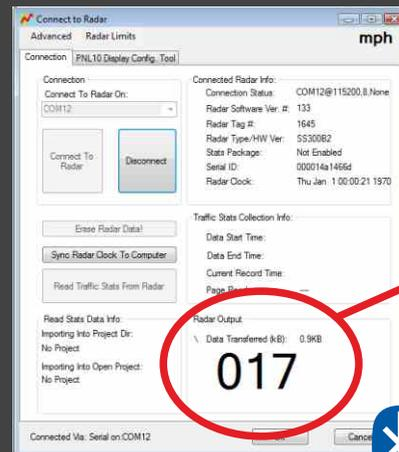
Constantly updating speed output transmitted to the remote computer via optional Bluetooth signal.
